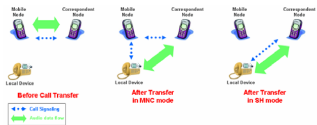
Figure 3-2: Transferring an only audio call to a local device in two different session transfer modes
